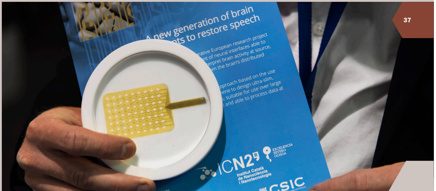
Flexible arrays of graphene solution-gated field effect transistors can be used to monitor brain activity. Credit: Alexandra Csuport
